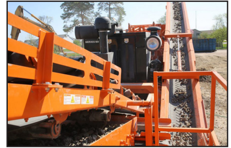
Top-deck retained material is returned to the crusher for further processing.
