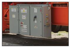
Includes removable electrical control panel featuring pre-wired receptacles for radial stackers.
