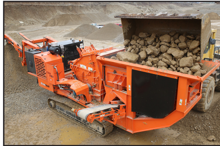
Heavy duty hopper-construction sized for feeding with a loader or excavator.
