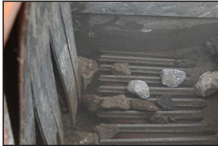
Grizzly bypass chute allows for either removal of the material that passes the grizzly deck onto a conveyor for stockpiling or for blending with the crushed material.
