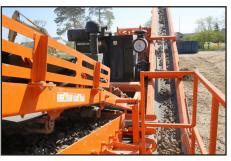
Top-deck retained material is returned to the crusher for further processing.
