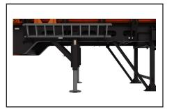
Hydraulic lift and leveling system enables quick set up and tear down by using the hydraulic run-on legs.
