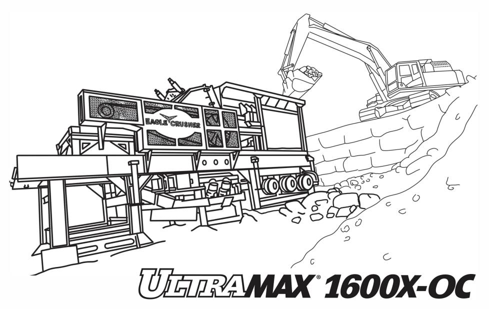
When concrete is recycled, it can still have metal, called rebar, inside in the concrete. That's why some crushers have MAGNETS on the conveyors - to separate the crushed concrete from the rebar.
