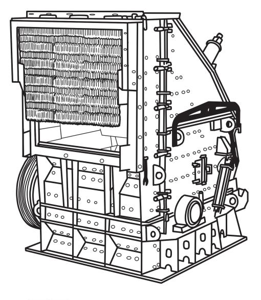
Many materials can be crushed using an IMPACTOR. An impactor's rotor can spin around hundreds of times per minute. The rocks collide with the rotor, fracturing it down into smaller pieces.
