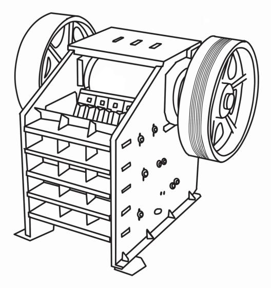
Another way materials can be broken down is by using a JAW crusher. Jaw crushers squeeze the material together with a lot of force until it breaks. Once the material is small enough it can pass through the bottom.
